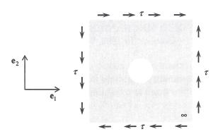
b. Determine the location of the highest principal stresses when the plate is subjected to a remote shear stress  $\tau$ . What is the value of the stress concentration factor (defined as the ratio between highest principal stress and  $\tau$ )?
